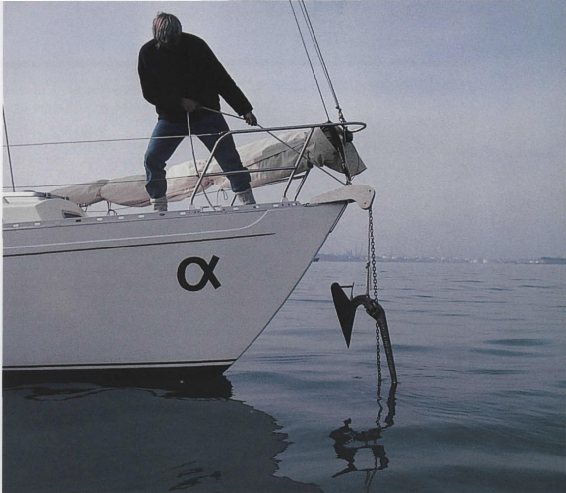
Capsizing a fouled anchor with a tripping line.
