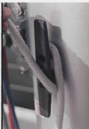
Making fast to a cleat. Note that this halyard cannot possibly jam and the coil is hung neatly and securely.
