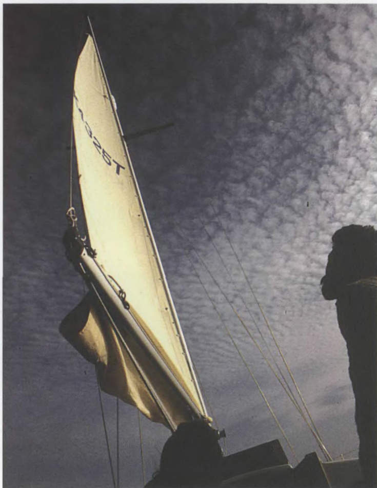
Mainsail twist is controlled by sheet and boom vang, or kicker.
