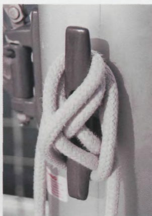
Making fast to a cleat. Note that this halyard cannot possibly jam and the coil is hung neatly and securely.
