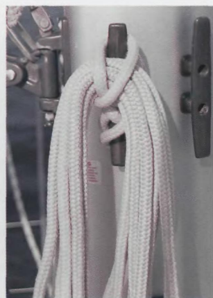
Making fast to a cleat. Note that this halyard cannot possibly jam and the coil is hung neatly and securely.
