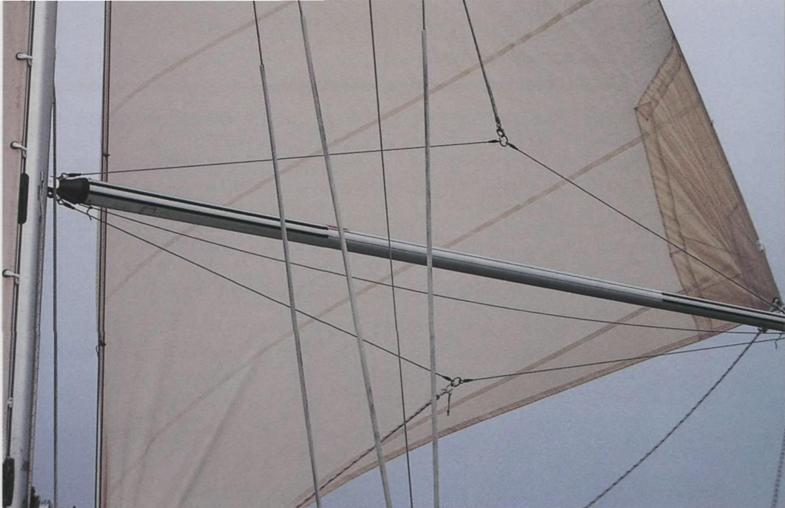
A genoa poled out on the run. Note topping lift and foreguy both rigged.
