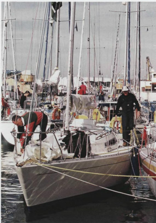
Rafting up: securing alongside a boat that is already fast to the dock, use bow line, stern line and springs to the other boat. When all is stable, run shore lines from your bow and stern to the dock and make sure you are taking your own weight – and always ask permission first.
