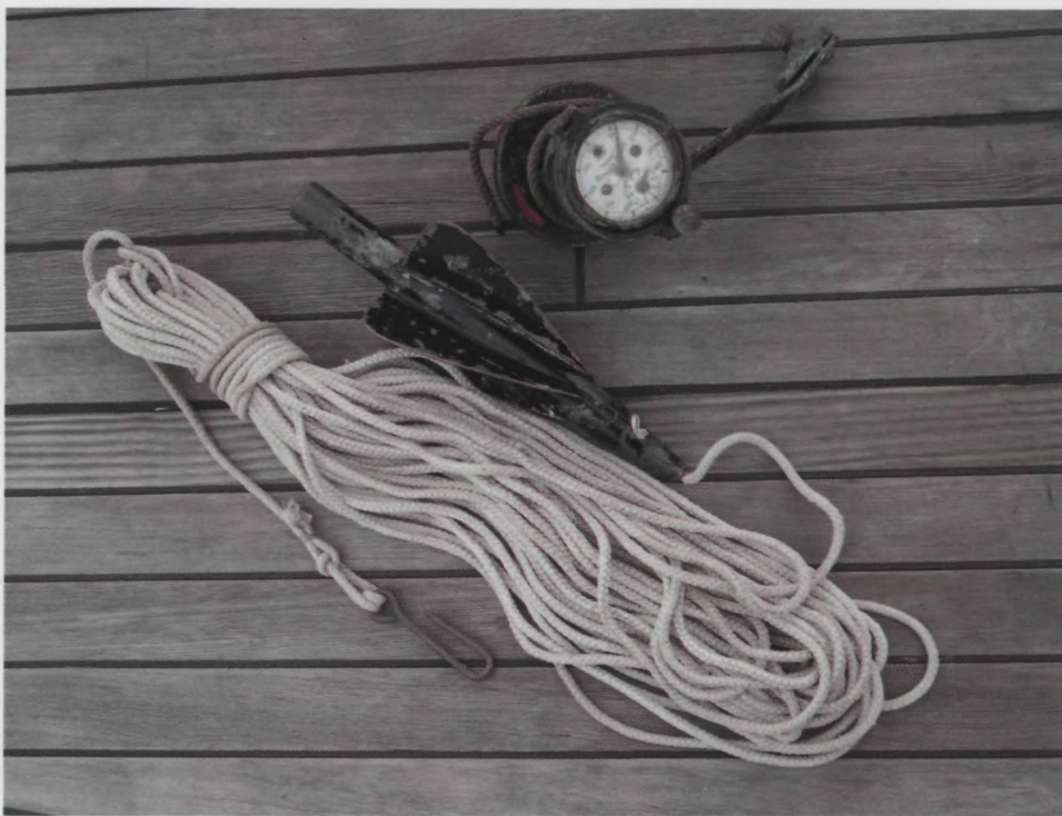
An old-fashioned trailing log is as near bullet-proof an instrument as you'll find.
