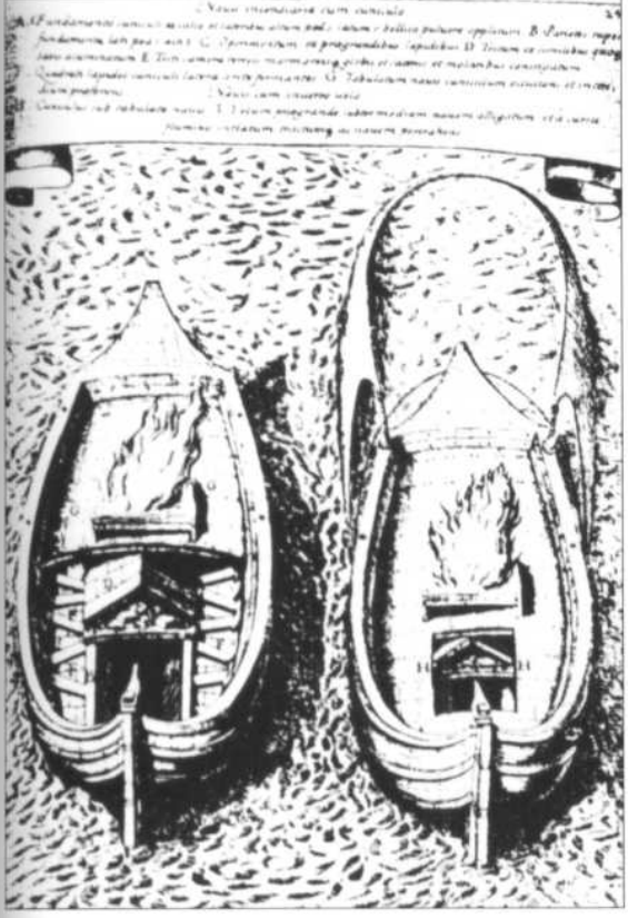
Fireships such as these were used decisively during the attack on the Spanish Armada off Calais on 7 August, 1588. The holds of small fishing vessels were filled with dry wood and pitch, then set alight by crews who first aimed the vessel towards the enemy before swiftly abandoning ship. Engraving from a maritime manual of 1590. (Mariners)
