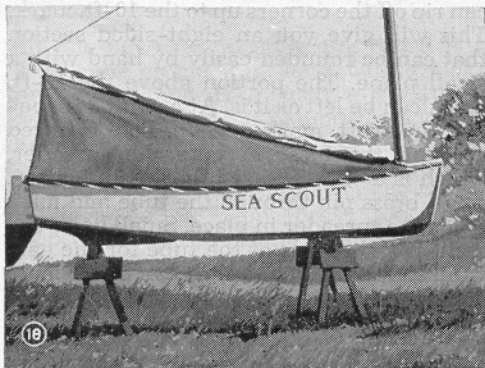
A tent cover, Figs. 18 and 19, is quite simple to make and is a protection to the boat and occupants when making cruises. The edges of the tent are held down by screw eyes spaced 8 in. apart below the boat's molding
