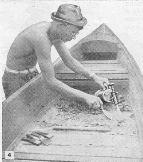
When refinishing, pay special attention to the inside of the boat. Damaged paint should be loosened with a blowtorch and scraped to expose bare wood
