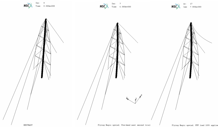
Figure 15: on the left the geometric model, in the middle the model under only pre tension and the final deformed structure on the right.
