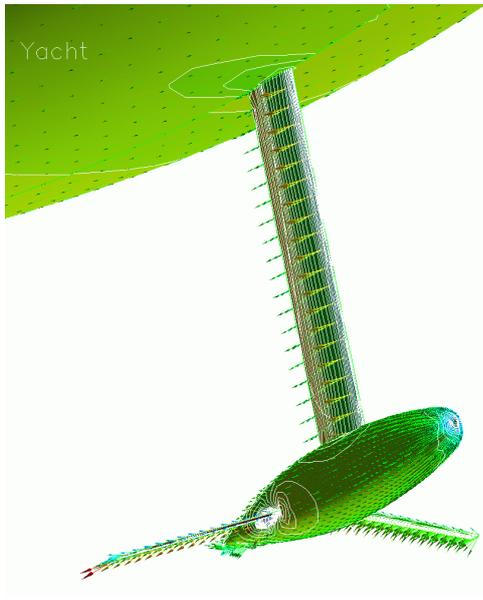
FIGURE 13: Perspective view of a simplified keel-bulb-winglet configuration featuring velocity vectors and pressure contours from a potential flow calculation
