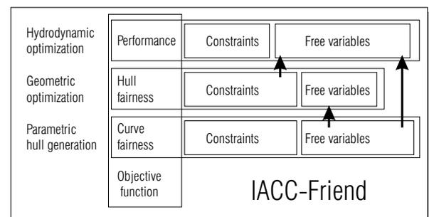
FIGURE 1: Levels of the hydrodynamic modeling system
