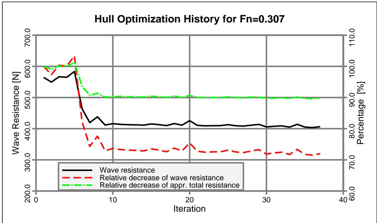
FIGURE 15: Optimization history for the canoe body without heel and leeway at  $F_n = 0.307$
