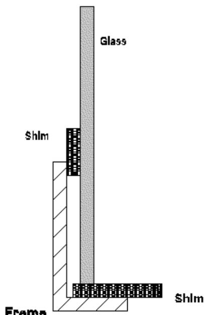
After the shims are in place, pull the glass back out and apply the bedding. Then set the window back into the bedded frame.
