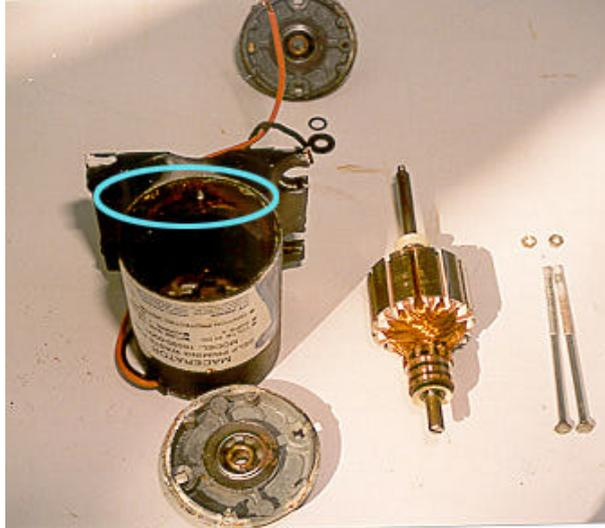
**Dismantled view of motor. The circled area denotes area of heavy corrosion that was inhibiting the motor rotation. Once cleaned up, the motor ran freely.**
