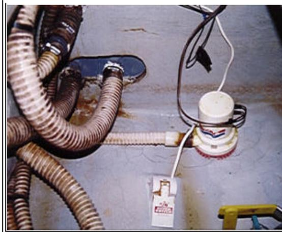
**How not to install a bilge pump. You can see by the high water line that it has already failed. The hoses at left were restraining the float switch and the wire connections were laying in the bilge water. They were moved prior to taking this photo. The builder installed it this way.**
